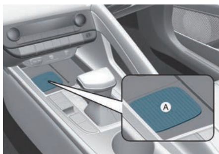
[A] Vehicle authentication pad (Wireless charging pad)
