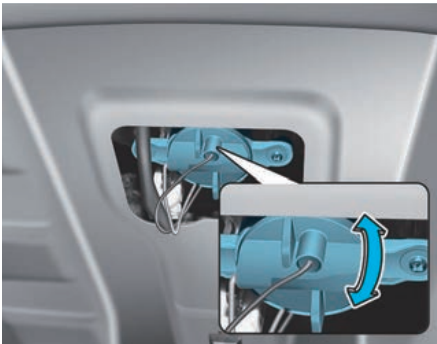
[A] High mounted stop light
