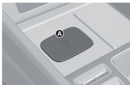
[A] Vehicle authentication pad (Wireless charging pad)
